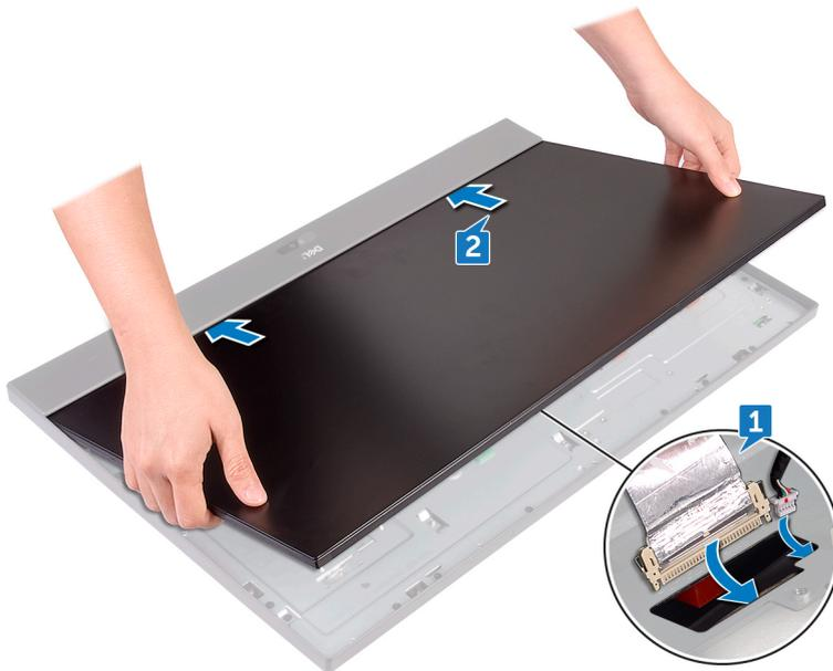
4. Connect touch-screen cable (TOUCH1) to the system board.
