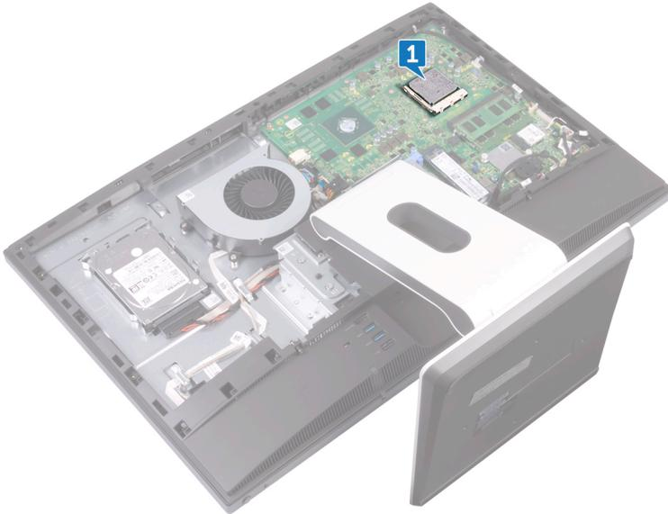
2. Press the release-lever down and then pull it outwards to release it from the securing tab.
