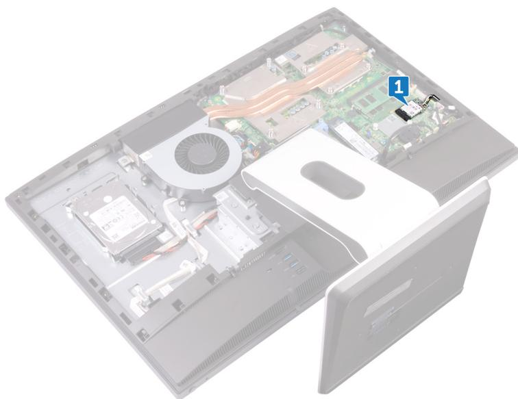
2. Remove the screw (M2x3.5) that secures the wireless card to the system board.
