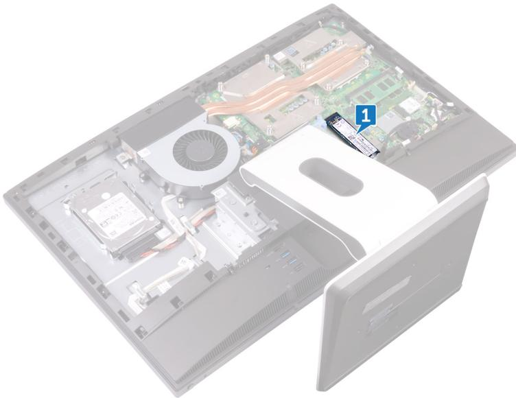
2. Remove the screw (M2x3.5) that secures the solid-state drive to the system board.
