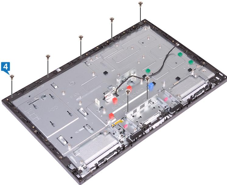
5. Route all the cables through the routing guides on the middle frame.
